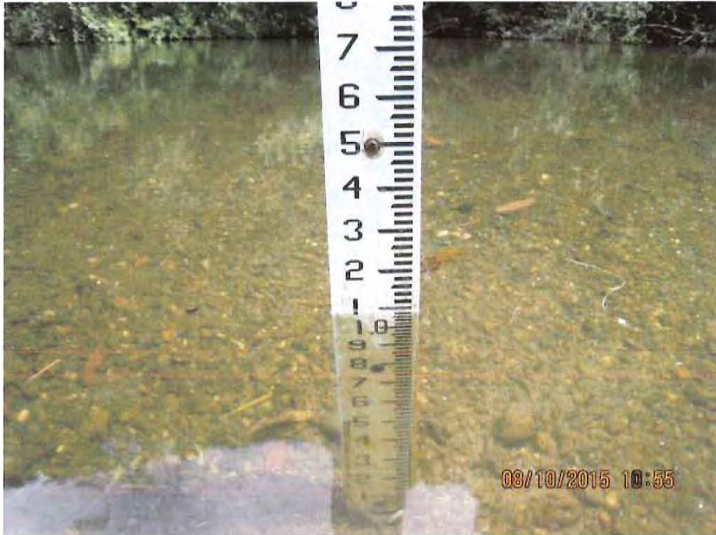
Photo 7305 0 ' Up Dir Pool Cr Station 0 LWD Site 0 08/10/15 10:55 AM Road# 40.1961 Mi. 0.1 Map Pt. 2156 THP Maintenance This is the pool gage when the water truck stopped pumping. There was no change.
