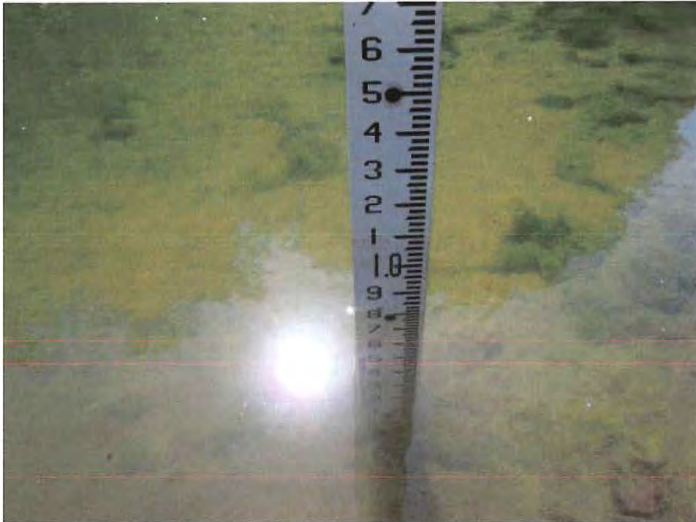
Photo 7366 36,557 ' Up SF Gualala Dir 0 Cr Station 0 LWD Site 0 09/02/15 3:19 PM Road# 40.09 Mi. 0.25 Map Pt. 2061 THP Huckleberry Nine minutes after the end of pumping, the water hight in the pool is still 0.85".
