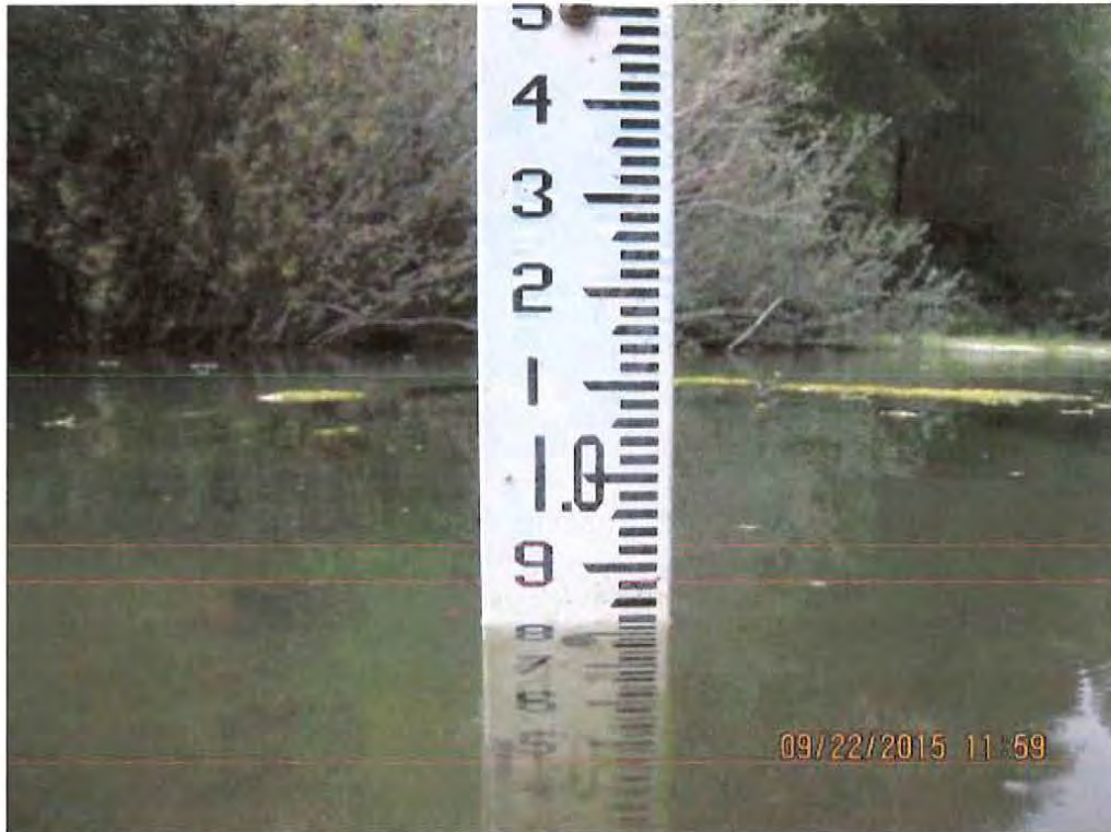
Photo 7413 0 ' Up SF Gualala Dir Pool Cr Station 0 LWD Site 0 09/22/15 11:59 AM Road# 40.09 Mi. 0.25 Map Pt. 2061 THP Huckleberry Ten minutes after the end of pumping the gage is still at 0.84'.
