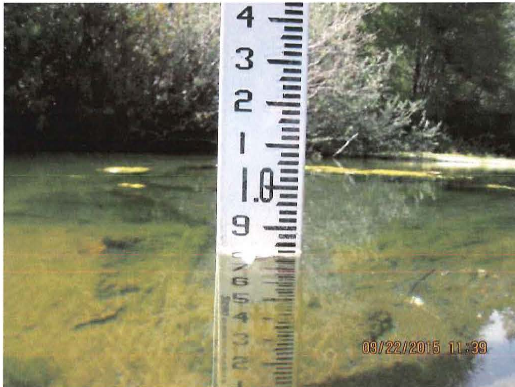
Photo 7410 0 ' Up SF Gualala Dir Pool Cr Station 0 LWD Site 0 09/22/15 11:39 AM Road# 40.09 Mi. 0.25 Map Pt. 2061 THP Huckleberry After seven minutes of pumping the gage is still at 0.84'.
