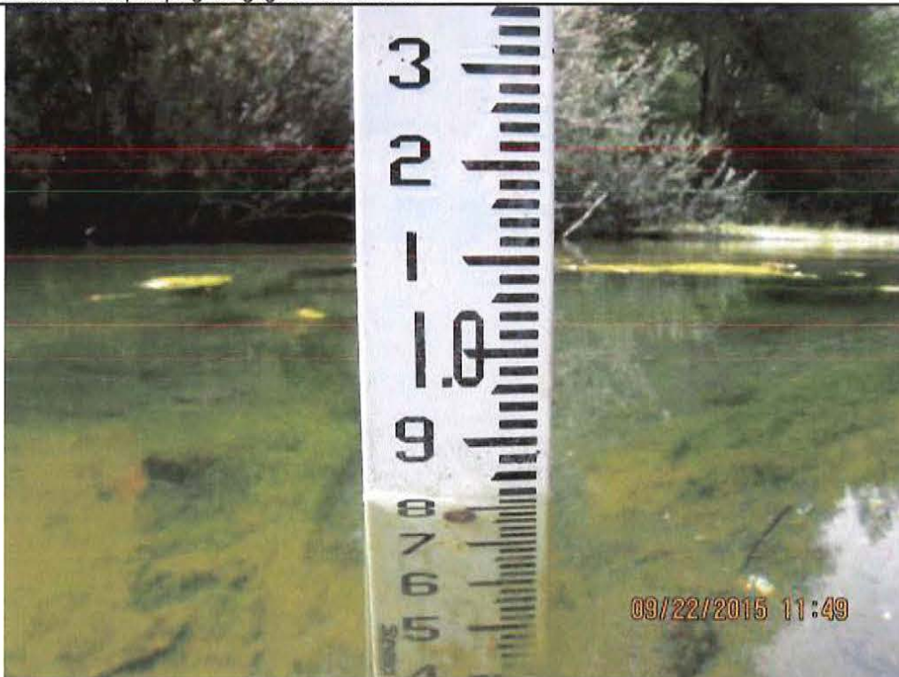
Photo 7411 0 ' Up SF Gualala Dir Pool Cr Station 0 LWD Site 0 09/22/15 11:49 AM Road# 40.09 Mi. 0.25 Map Pt. 2061 THP Huckleberry After sixteen minutes of pumping the gage is still at 0.84'.
