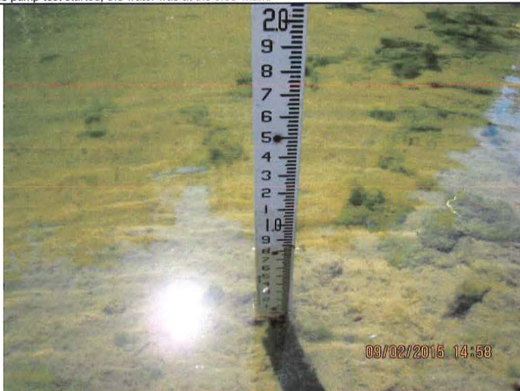
Photo 7363 36,551 ' Up SF Gualala Dir 0 Cr Station 0 LWD Site 0 09/02/15 2:58 PM Road# 40.09 Mi. 0.25 Map Pt. 2061 THP Huckleberry Pumping started at 2:56 pm. The water height is still 0.85'.
