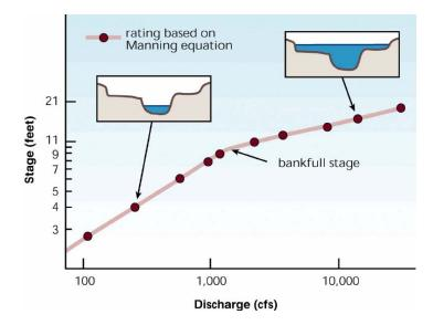
Figure 6. Hypothetical stage-discharge relationships for both the main river channel and for the floodplain surface. Bankfull stage can be determined from this rating curve [Figure 7.4 in Stream Corridor Restoration, FISRWG (1998)].
