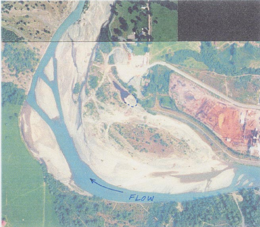
1996 photo of Blue Lake Bar wetland pit excavated in 1993 and enlarged in 1994. Pit has partially re-filled with marketable aggregate (dashed line indicates original pit boundary).
