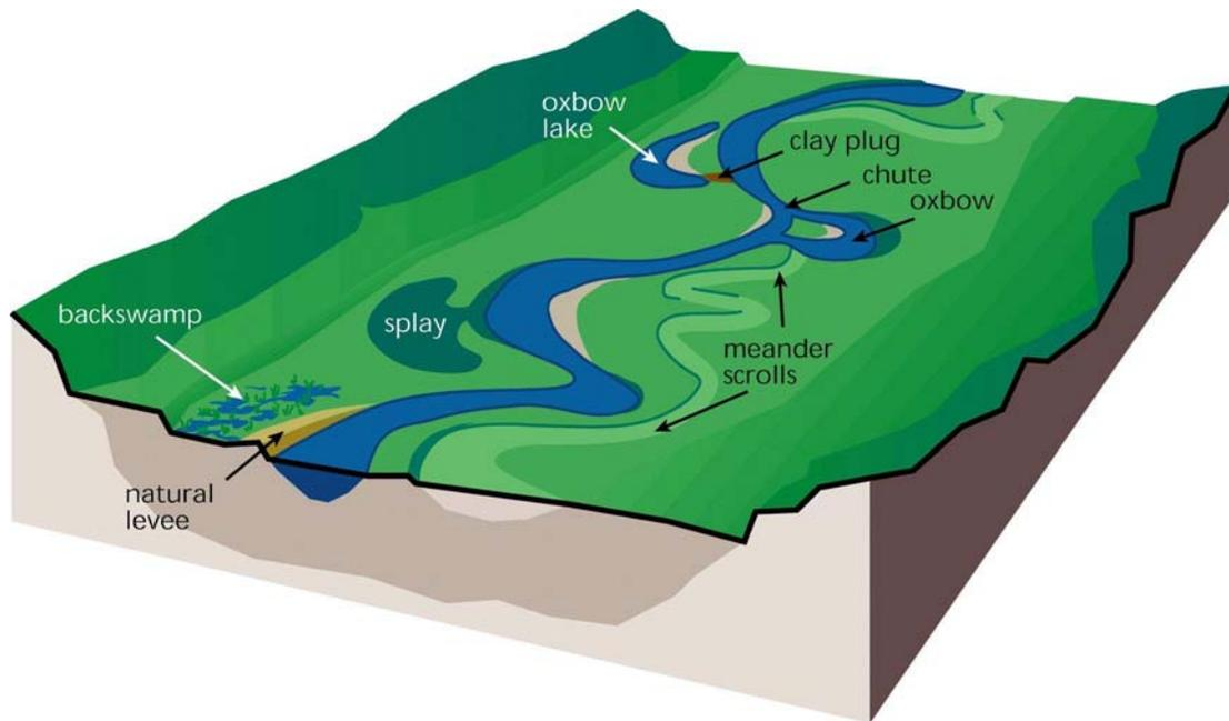
Figure 13. Diagram showing the formation of an oxbow lake on a floodplain [Figure 1.21 in Stream Corridor Restoration, FISRWG (1998)].
