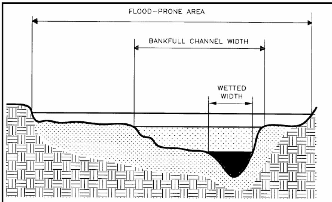
Figure 5. Diagram of stream channel and flood prone area cross-section (Figure III.1 in California Salmonid Stream Habitat Restoration Manual, Third Edition; [Flosi and others 1998]).
